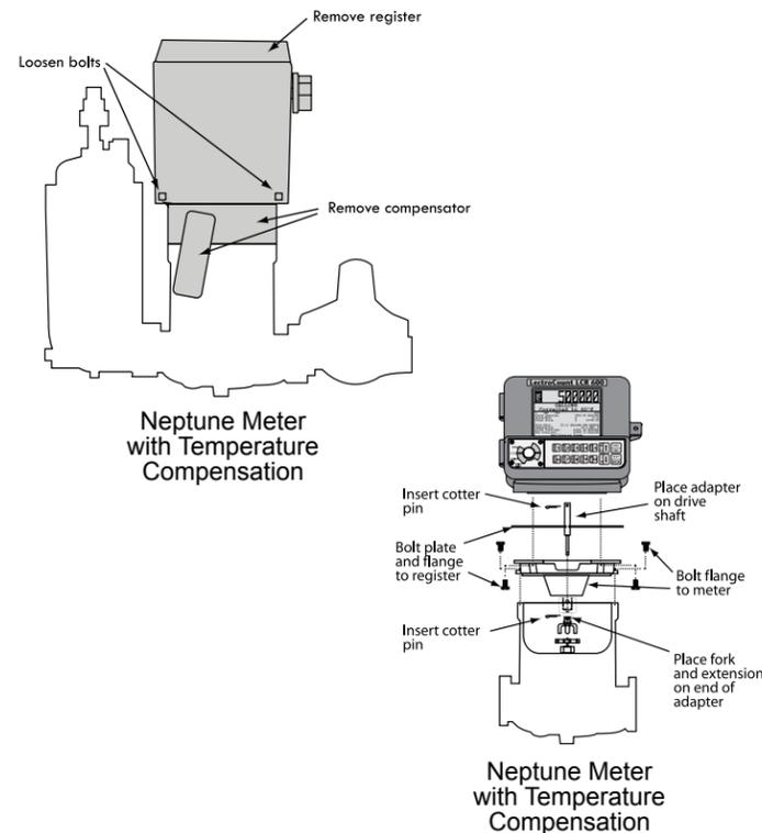
Installation kits 82641 (E-26 series) & 82642 (E-36 series) are specifically designed for previously temperature compensated Neptune meters.
