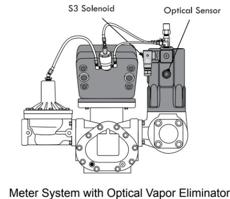
**To wire optical air and vapor eliminators to the LCR 600:**
