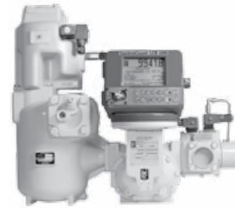
M7 Meter with LectroCount LCR 600 Electronic Register, Optical Air Eliminator, High Capacity Strainer, and E-7 Valve
