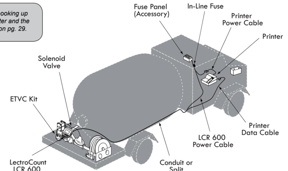
**Electronic Temperature Volume Compensation (ETVC) Installation**
