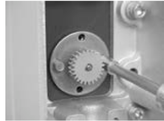
Remove Packing Gland Mounting Screws
